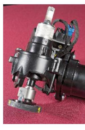
Below: The EZ power steering unit is compact and either sits under the dashboard, or in the case of the 911, in the 'smuggler's box' in the front luggage area. The steering can be set up for differing levels of assistance Left: EZ Electric Power Steering main man, Roger Reijngoud
