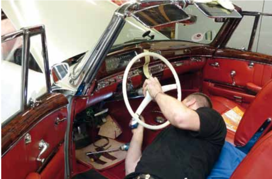
The Ponton cabriolet steering column loosened ready for extraction.
