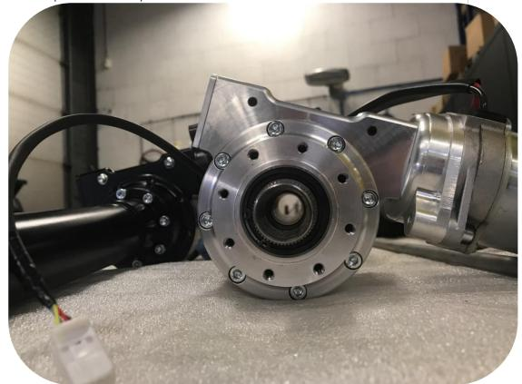
The system can be supplied as a kit with adapters that allow mounting the unit in the original steering column. For several models, we supply a complete replacement column. In most cases, it is possible to restore the original steering system to its original condition.
